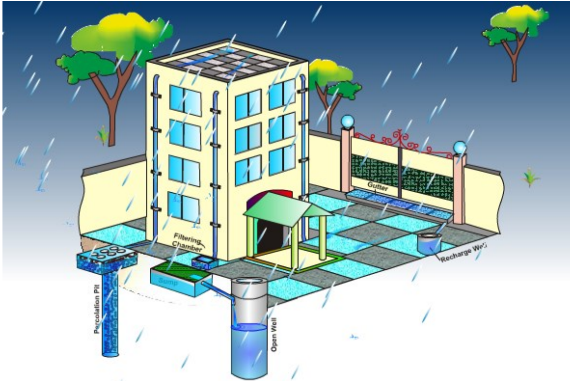
Rainwater Collection in Multistoried Roofs
